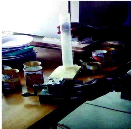
Plate 1: Tapping apparatus
