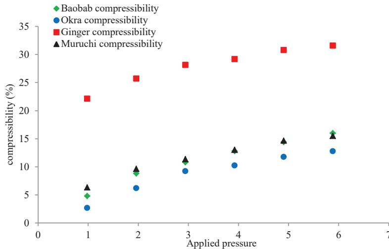
Figure 3: the plots of compressibility against applied pressure for baobab, okra, ginger, and muruchi powders
