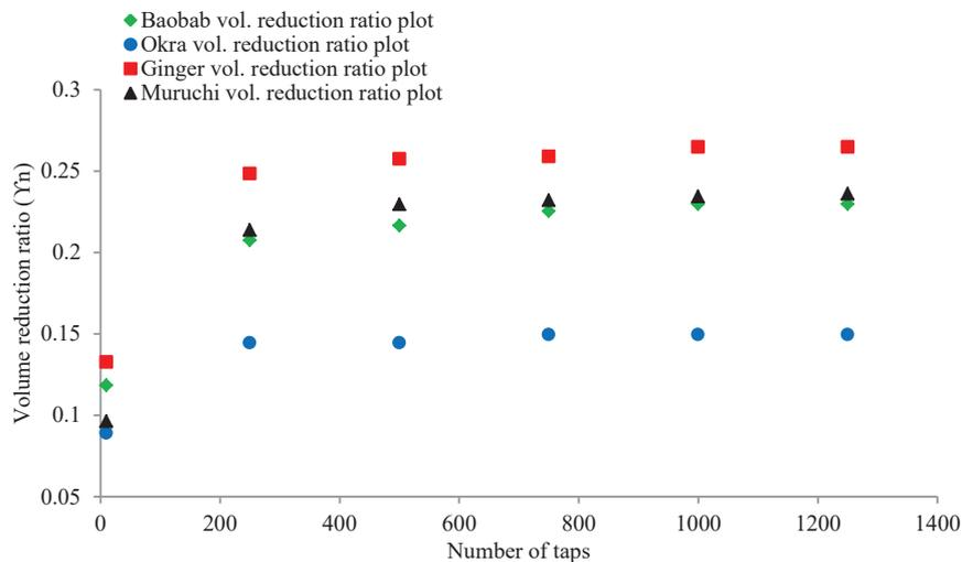
Figure 1: the plots of volume reduction ratio against number of taps for baobab, okra, ginger and muruchi powders
