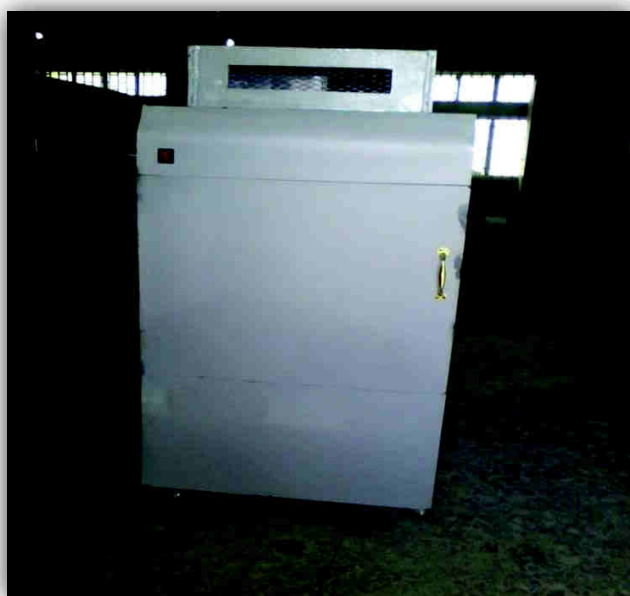
Fig. 1: The Dryer Showing the Drying Cabinet.
