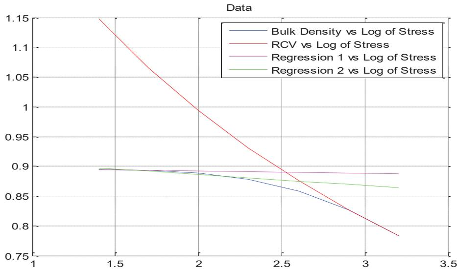
Figure 5: Graphical Interface for Estimating Pre-compression Stress for the Ire set of data
