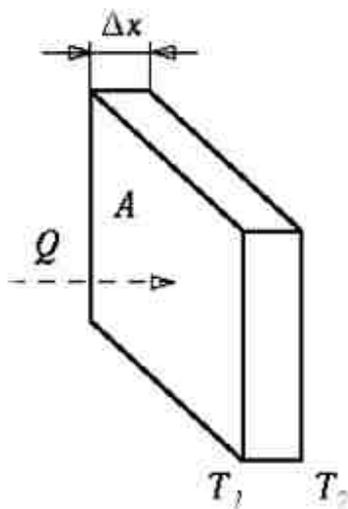
Figure 2. Heat transfer process through surfaces with different temperature
