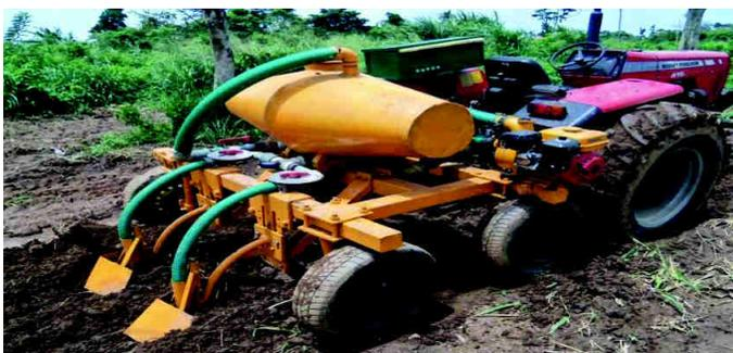
Figure 6: Liquid manure injector equipment
