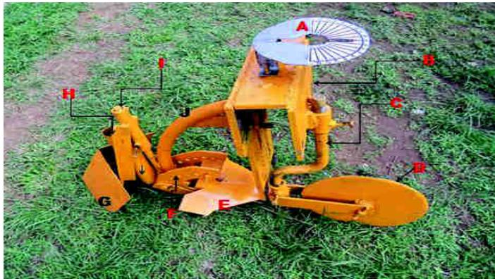
Figure 1: Manure injector components
