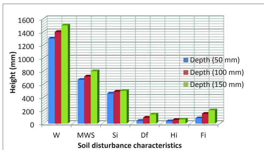
Figure 7: Soil surface disturbance characteristic/depth at 3.49 km/h speed using CS<sub>wc</sub>
