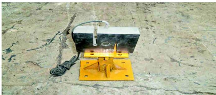
Figure 3: 20-ton Load cell
