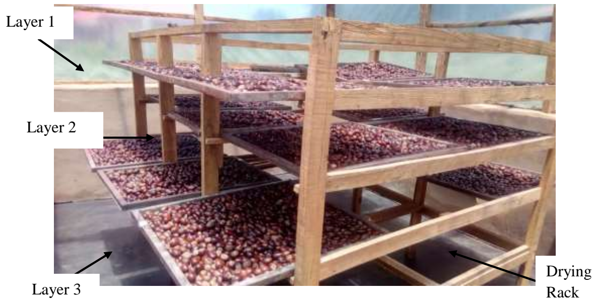
Figure 3a: Samples of Shea Nut being Dried on Different Layers in the Dryer
