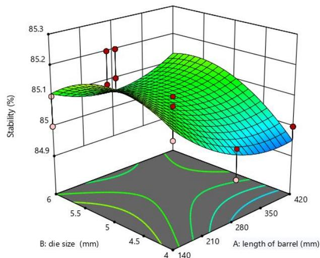
Figure 2: Effect of length of barrel and die size on the water stability
