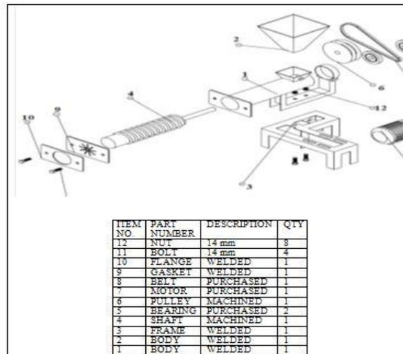
Figure 2: The Exploded view of the Pelleting Machine
