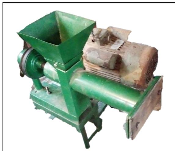
Figure 3: Pictorial view of the Fabricated Pelletizing Machine
