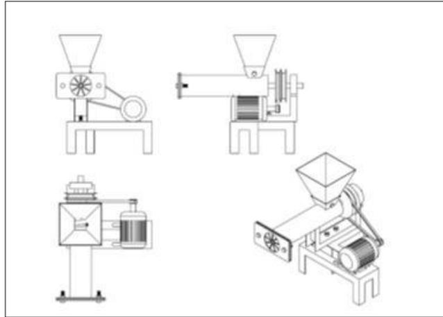
Figure 1: The Isometric view of the Pelleting Machine
