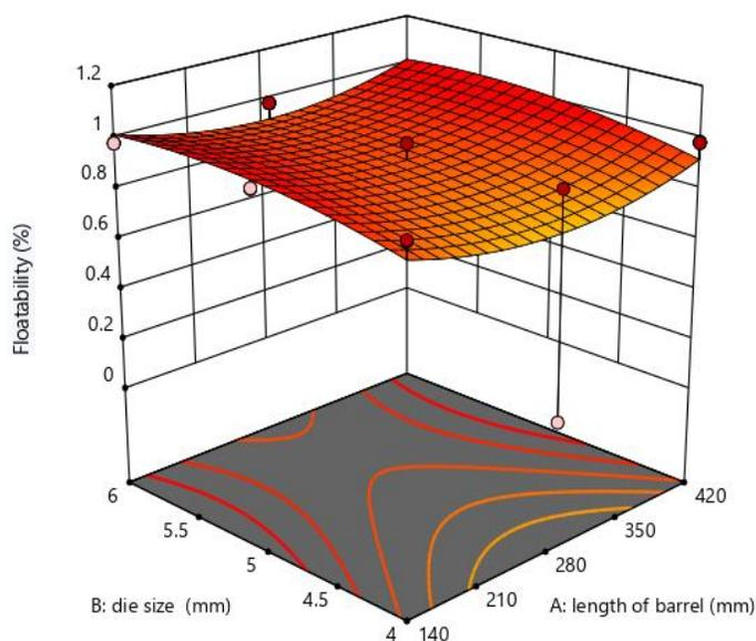
Figure 3: Effect of length of barrel and die size on the floatability
