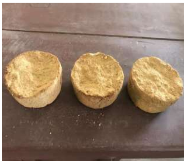
Figure 3: A set of three briquettes used in the filter columns
