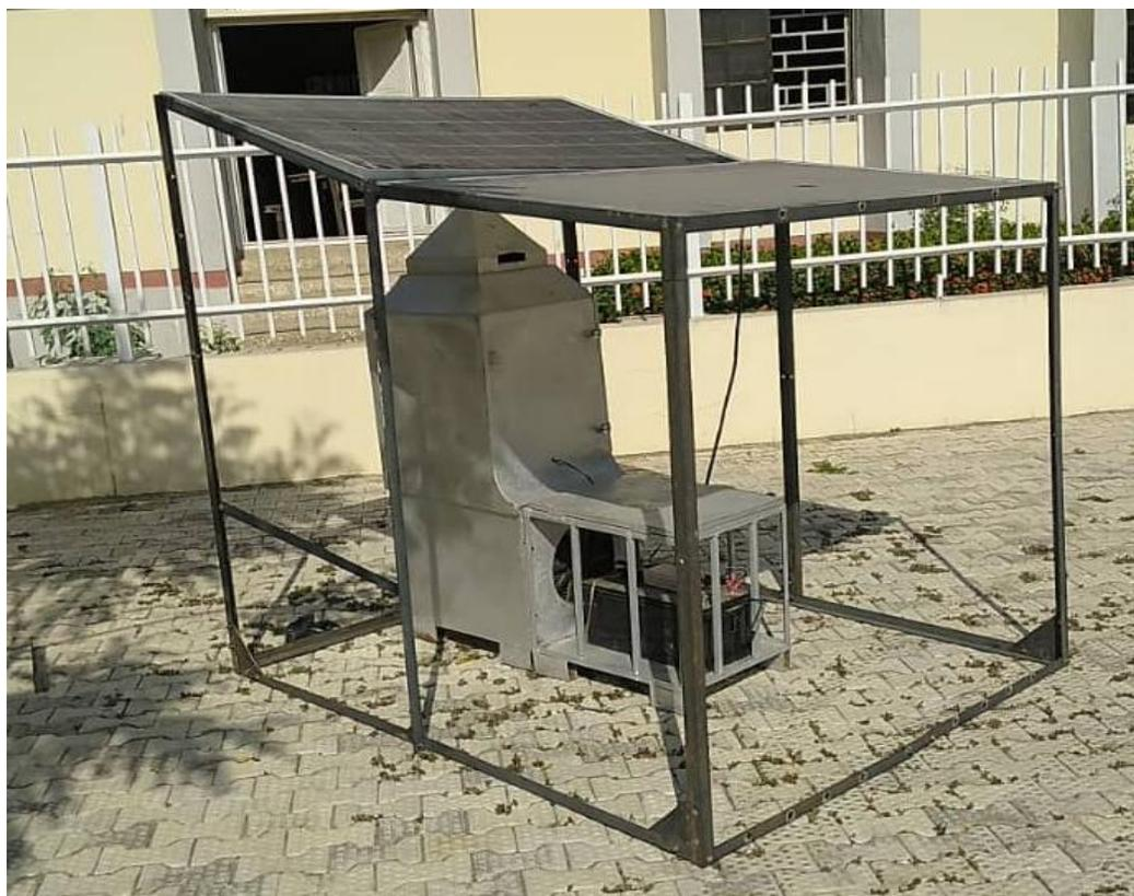
Figure 2: Photo of the continuous drying solar dryer
