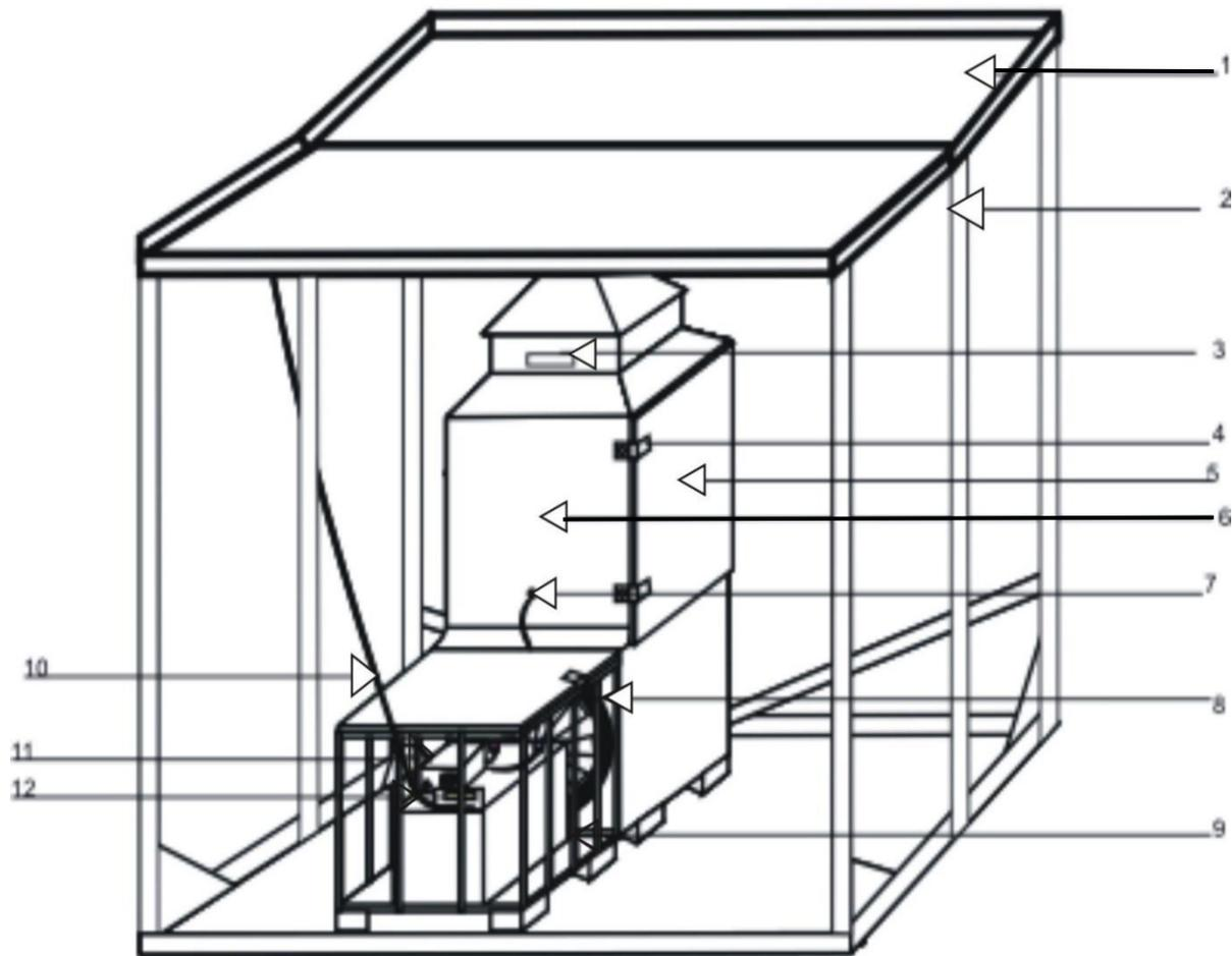
Figure 1: Continuous drying solar dryer showing the working components
