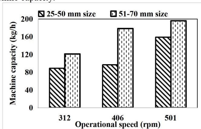
Figure 4: Variations in machine capacity with operational speed
