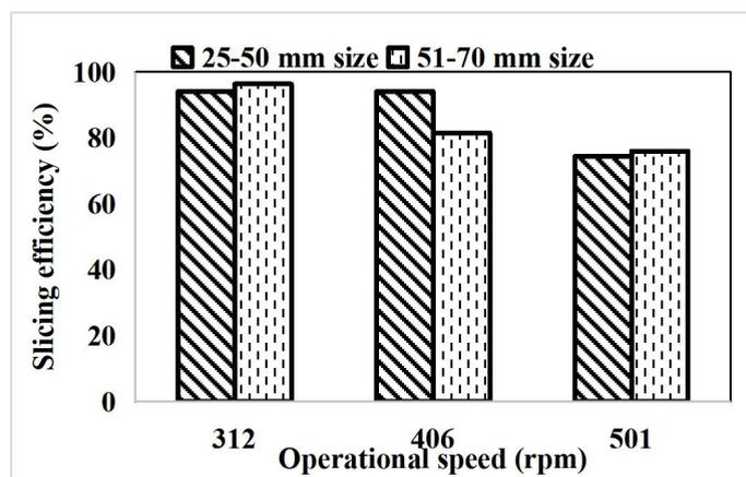
Figure 3: Variations in slicing efficiency with operational speed
