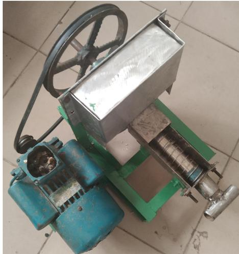
**Figure 2: Fabricated portable potato slicer**
