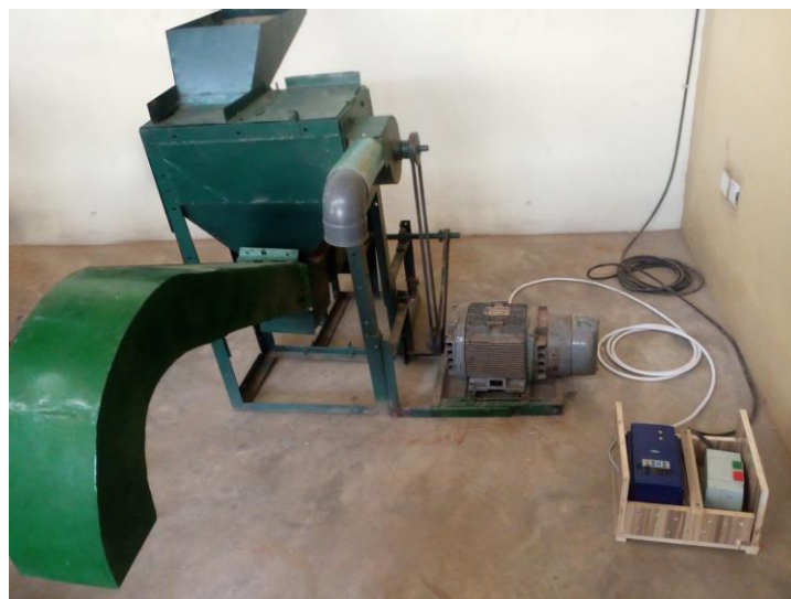
Figure 3: The fabricated Soybean thresher
