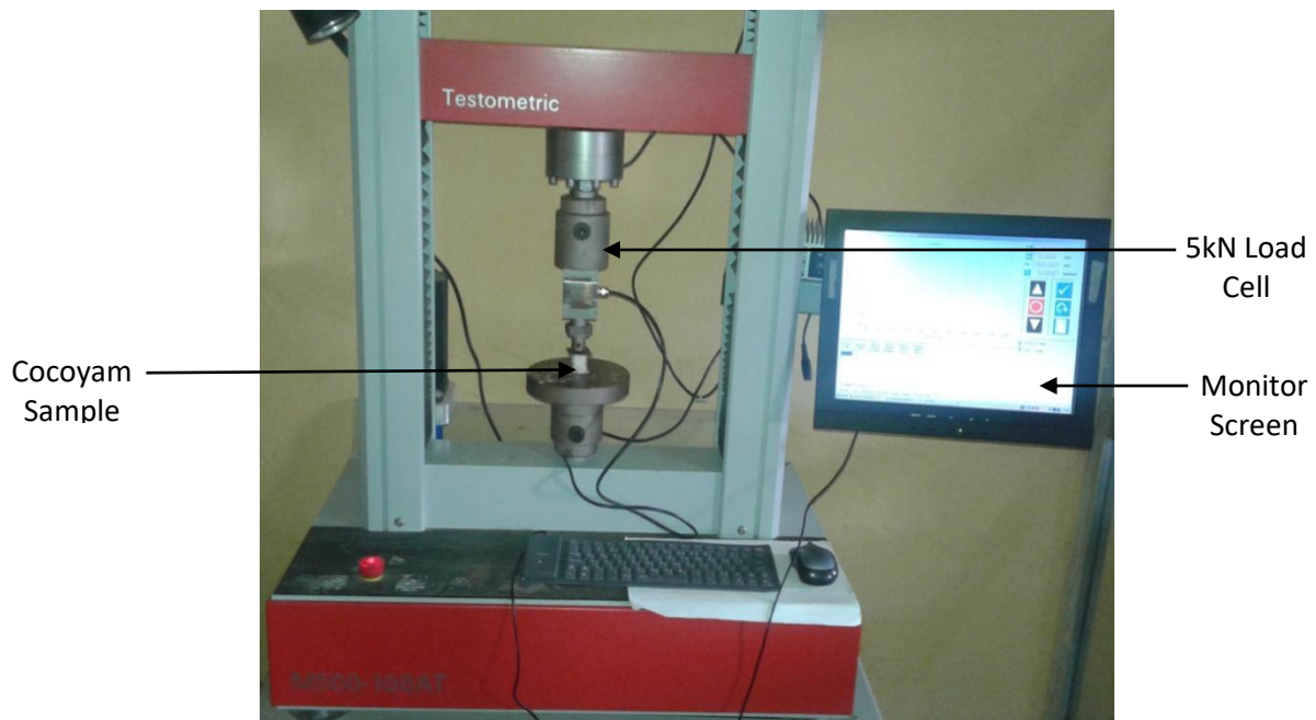
Figure 1: Experimental Set-up for Determination of Mechanical Properties of Cocoyam Cormel
