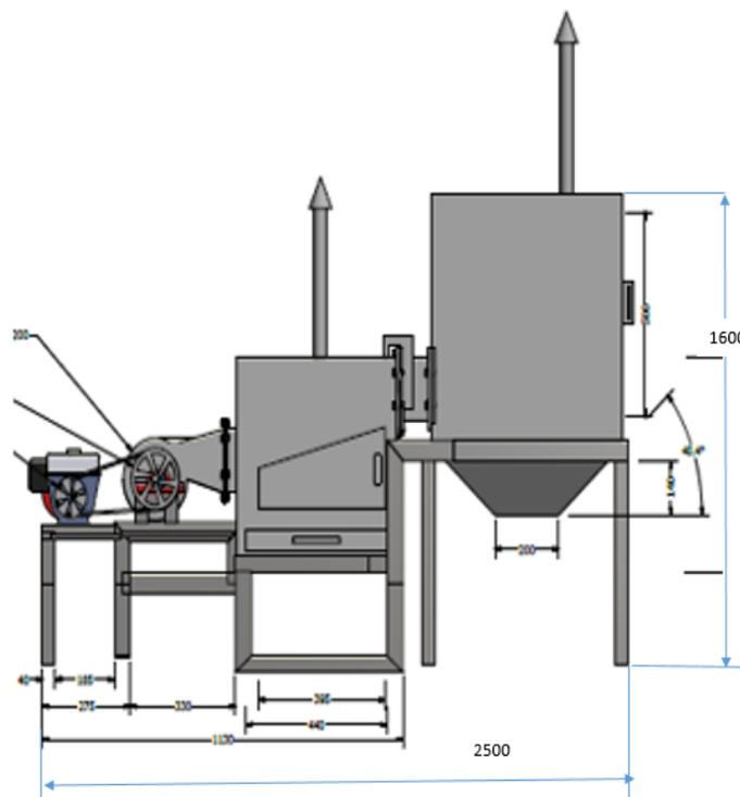
**Figure 2:** Pictorial View of the Biomass-fired force-convection cabinet drier
