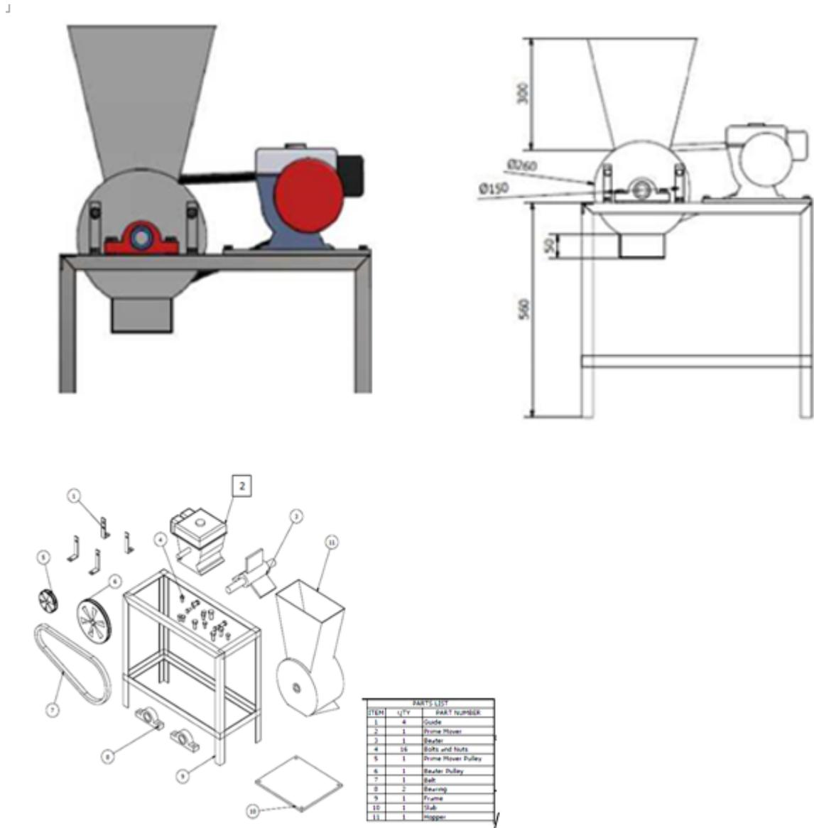
**Figure 3:** Pictorial (Front elevation) and Exploded views of the Centrifugal Impact Palm Nut Cracker
