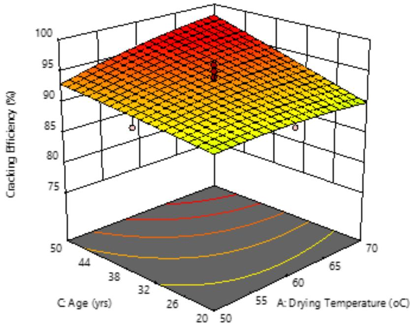
**Figure 4:** Surface Response 3D plot showing the effect of the age of the palm tree at the drying period of 21 h on the cracking efficiency.
