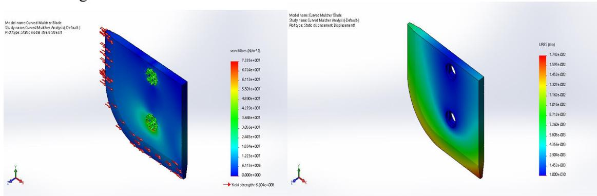
Figure 14: Maximum stress and maximum deformation for blade with 150° lifting angle
