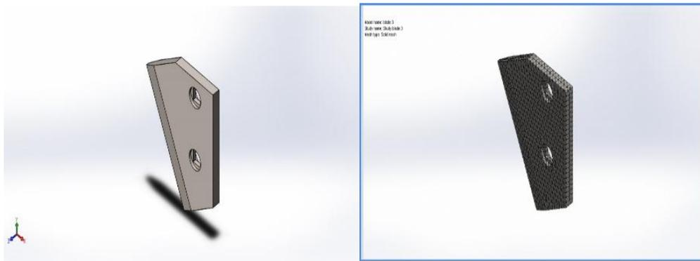
Figure 9: Geometric model and mesh density for blade with 120° lifting angle
