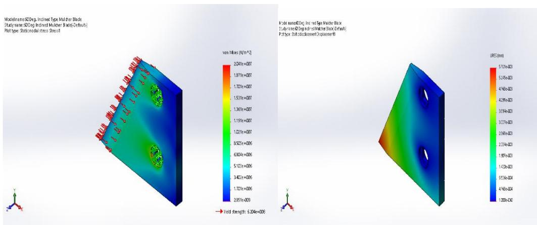
Figure 8: Maximum stress and deformation for blade with 60° lifting angle
