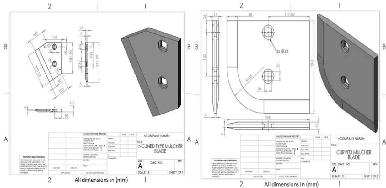
Figure 2: Orthographic and 3D Model Mulcher Blade with 120° and 150° Lifting Angle
