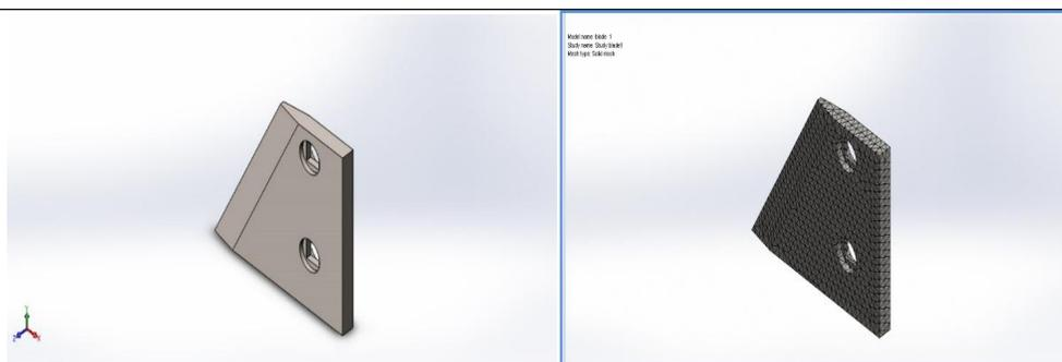
Figure 6: Geometric model and meshing density for blade with 60° lifting angle
