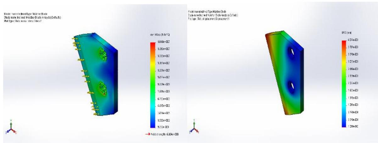
Figure 11: Maximum stress and maximum deformation for blade with 120° lifting angle
