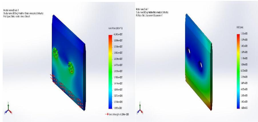
Figure 5: Maximum stress and maximum deformation for blade with 0° lifting angle
