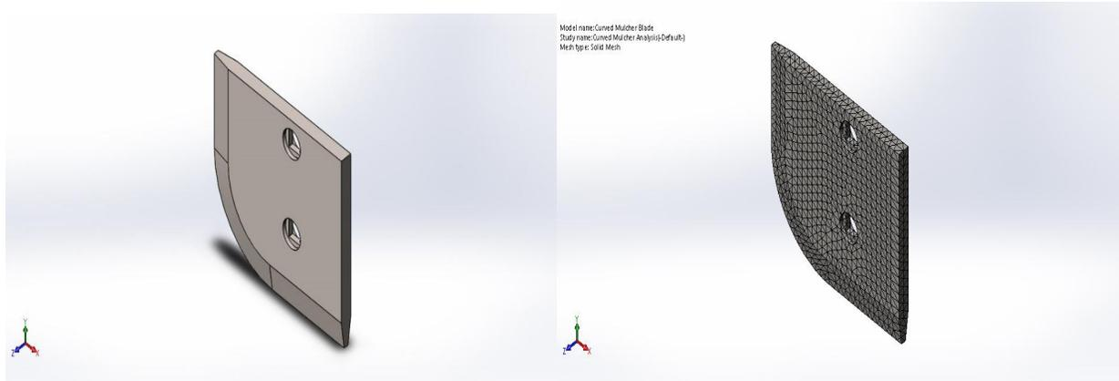
Figure 12: Geometric model and meshing density for blade with 150o lifting angle
