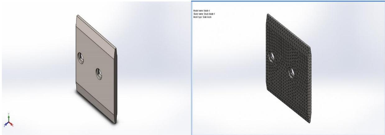
Figure 3: Geometric model and meshing density for blade with 0° lifting angle
