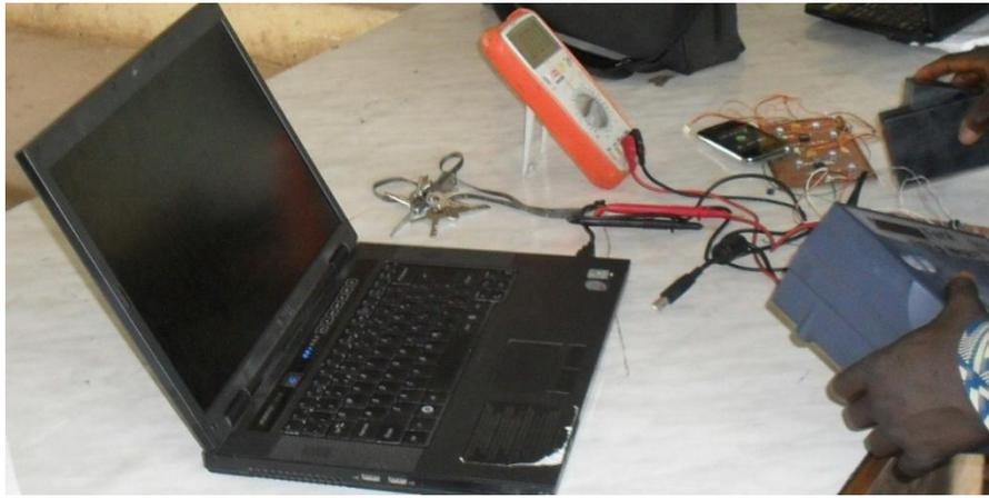
Figure 3: Aspect of the Instrumentation System showing the Computer System, Data Logger, Circuited Amplifier and the Voltage Meter during the Calibration Process
