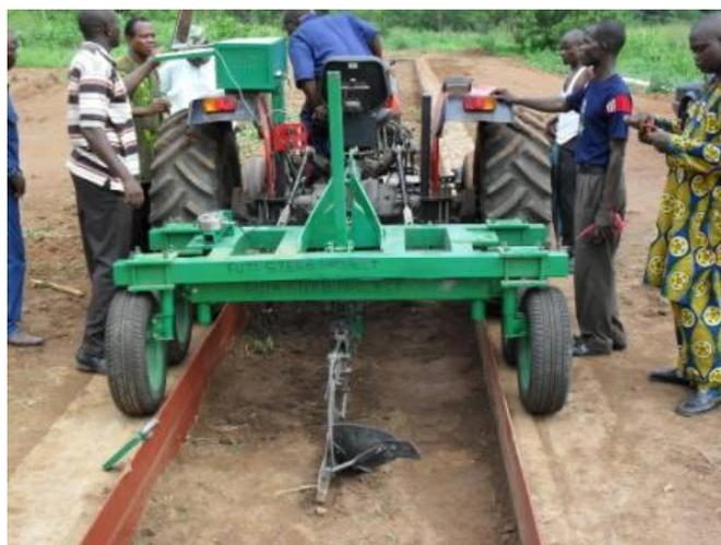
Figure 2: Implement Carrier and Drive System during the Trial Test of the Instrumentation System
