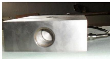
Figure 6: Load cell.
